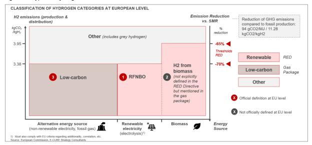
Figure 3 - Types of hydrogen
