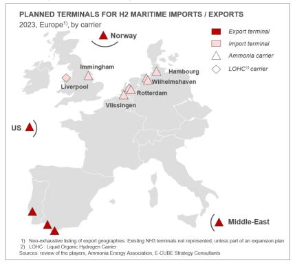
Figure 7 - H2 terminalling infrastructure under development
