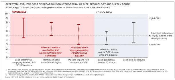
Figure 8 - Levelized costs of decarbonised H2 (under gaseous form) delivered in Western Europe
